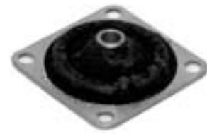
**ROUND MOUNT** - 1-1/4" overall length as used on Cessna aircraft. Rubber center is 1/2" x 9/16" with 8-32 threaded steel projections.
