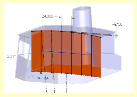
First, I sketched the vertical centerlines for the Bridge Divider wall's reinforcing studs, as show in the figure above. I used sketch symmetry, plus some horizontal construction lines (with EQUAL length relations), to enforce a desired 24" spacing on-centers. This wall is bounded by a curved roof plate, so I'll let the studs go all the way to the edge of the plate for now, (easier to sketch), but they will be trimmed later.
