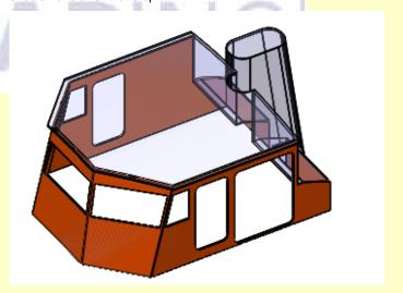
Next, let's get a separate solid body for the roof. You can see from the image above that the funnel shroud and the roof intersect such that there is a 'C' shaped notch at the back center of the roof. In the actual boat, that does not really happen. Most of the funnel shroud is cosmetic, and the roof in fact is unbroken along the aft edge. But our simplified master-solid Merged these two features – how do we get back to a clean, unbroken roof line?
