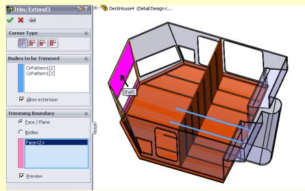
Using the same Trim/Extend command, we now trim the tops of all the wall stringers so that they terminate on the underside of the rafters we've just
