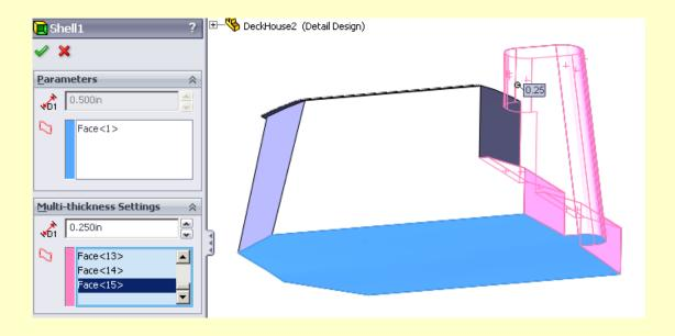
The last things to do before getting into fabrication details, are to cut thru the window and door outlines, and to make the entire body translucent, (I use a light color like yellow, or sky-blue, and a transparency of 85%). That way we can see to work on and reference the master body, but have most of our attention upon the (opaque) fabrication details as they take shape.
