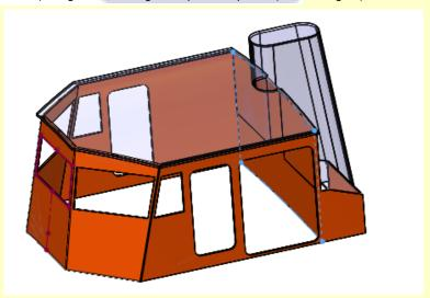
While we're at it, the large doorway (on the Port-side only), is for passengers fo go down stairs, so this is actually walled-off from the bridge. We could create this wall by first locating a point halfway between the larger and the
