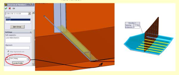
Again, using the 2.31-degree angle measured from sketching the prior stringers, we create the pattern of 6 rafters along the inside of the roof.
